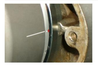
If you used the new rotor to turn the engine, carefully remove the rotor **without changing the position of the crankshaft!** With the engine still at ignition position, carefully replace the rotor on the crankshaft, aligning the timing mark on the rotor with the timing mark on the stator plate.
