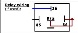
The brown wire with the ring terminal from pins 87a und 86 goes to ground.
