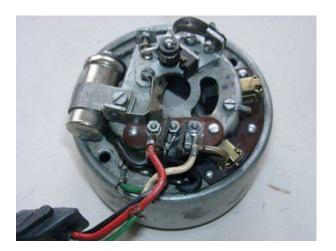
Losen all cables to the generator, regulator and ignition coil, then remove the generator with the regulator and ignition coil.
