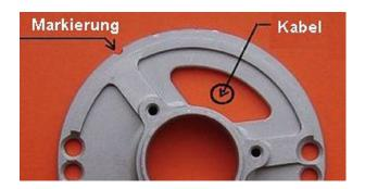
Take a look at the stator base plate (aluminium). You will find there, left from the cabel passage ("Kabel"), a small notch ("Markierung") on the circumference.
